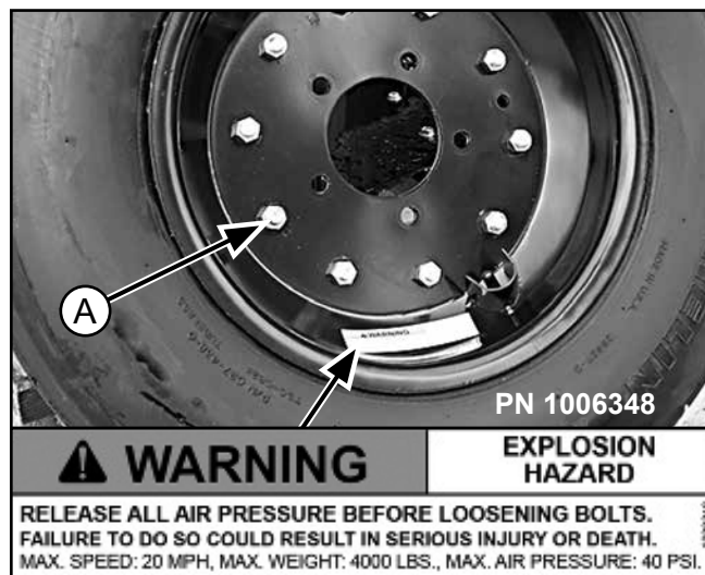
Figure 21. Split Rim Tire Servicing
