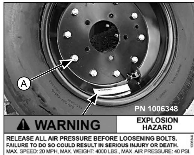
Figure 21. Split Rim Tire Servicing
