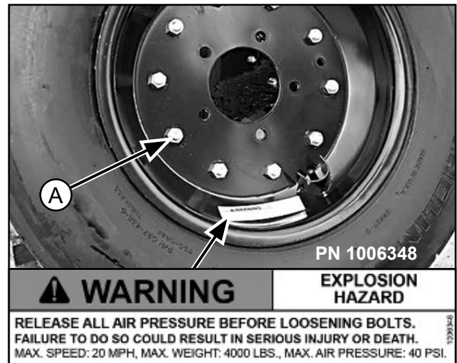
Figure 9. Split Rim Tire Servicing
