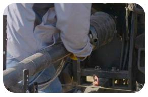
Once in position,the SmartLift™ holds the driveshaft while a spring allows for easy vertical adjustment.
