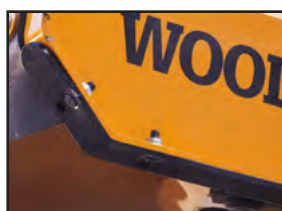
Optional bolt-on replaceable skid shoes for longer wear.
