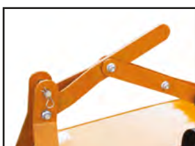
Breakaway link allows slasher to float and follow terrain for better cut quality.
