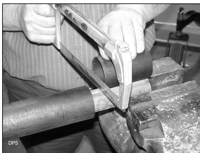
Figure 7. Cut Shaft to Length
