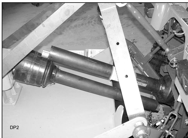
Figure 4. Drive Halves Placed Parallel
