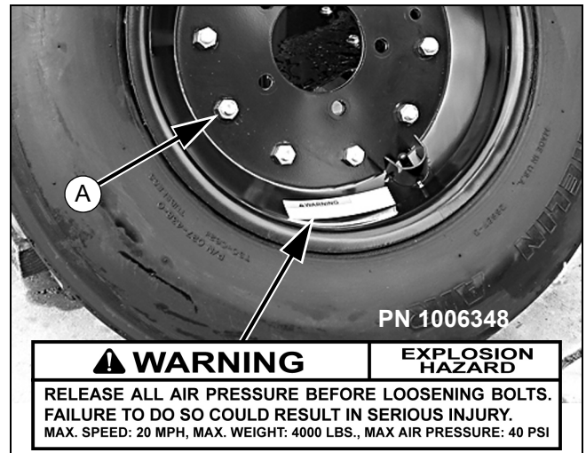
Figure 10. Split Rim Tire Servicing
