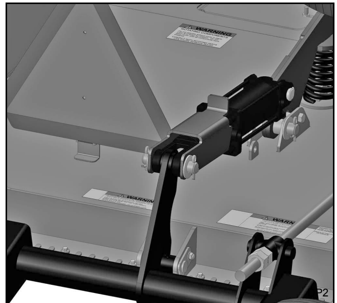
Figure 4. Transport Lock In Transport Position
