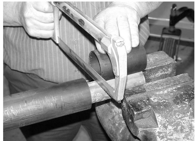
**Figure 4.** Cut Shaft to Length
