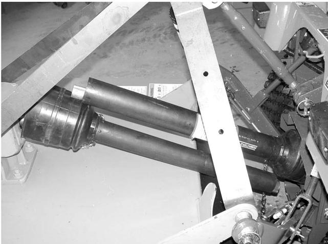
**Figure 1.** Drive Halves Placed Parallel
