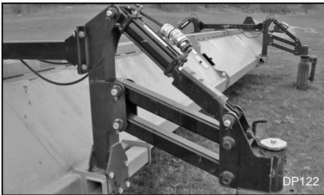
Figure 48. Pivot Tubes, Caster Pivots & Cylinders Installed
