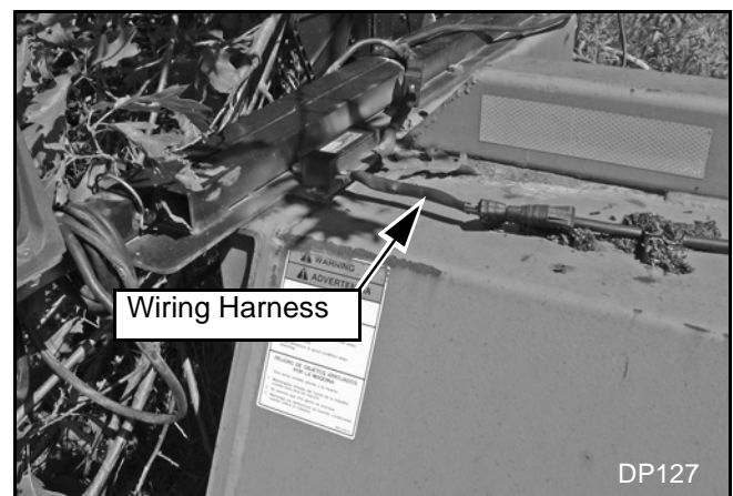
Figure 56. Safety Light Wiring
