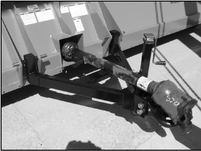
Figure 51. Pull-Type Hitch Installed
