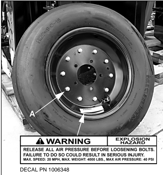
Figure 15. Split Rim Tire Servicing
